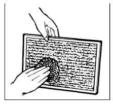
To clean grease filter, soak, then agitate filter in hot detergent' solution. Don't use ammonia or other alkali because it will darken metal. Highttbrushing can be used to remove embedded dirt. Rinse, shake and remove moisture before replacing. Filters should be cleaned at least once a month. Never operate your hood without the filter in place. In situations where flaming might occur on surfaces below hood, filter will retard entry of flames into the unit.
